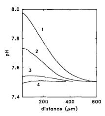
Fig. 3. A group of steady-state pH profiles near a BLM induced by acetate and ammonium permeation. The solution contained 1 mM Tris, 1 mM Mes, 100 mM choline chloride, pH 7.5. 30 mM ammonium nitrate were added to the *trans* side of the membrane. The concentration of sodium acetate at the *trans* side was varied: (1) no acetate, (2) 90 mM, (3) 190 mM, (4) 250 mM.
